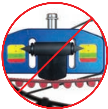
Too much belt tension
