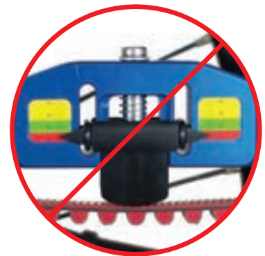
Too little belt tension
