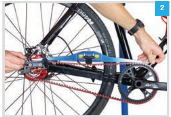
Contacting both sprockets, measure the belt tension across the span.
