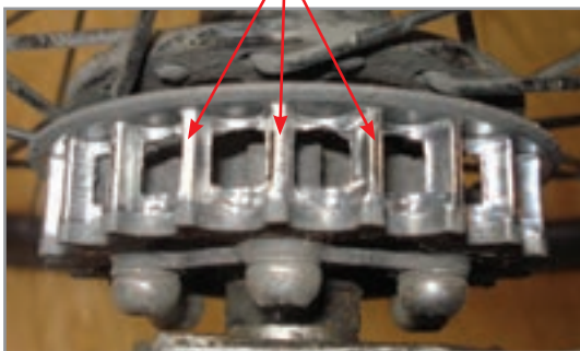
Worn CDC Sprocket Teeth
